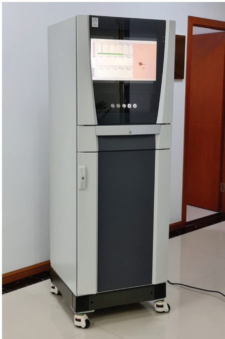
Algapro 21L, the online version for onsite phytoplankton monitoring
