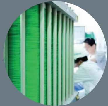
FIG. 11: An early electro-deionisation prototype module
