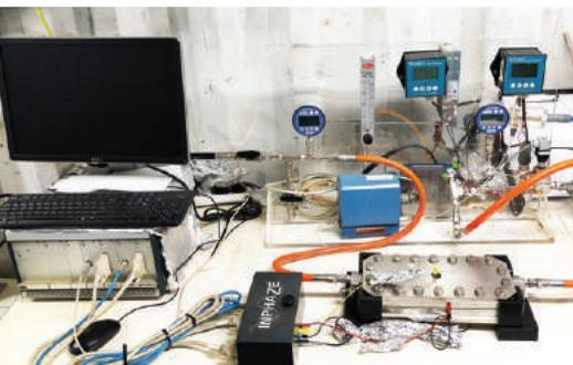
FIG. 1: Electrical Impedance Spectroscopy Fouling Monitor (EISFM) set-up at the pilot seawater reverse osmosis (SWRO) plant
