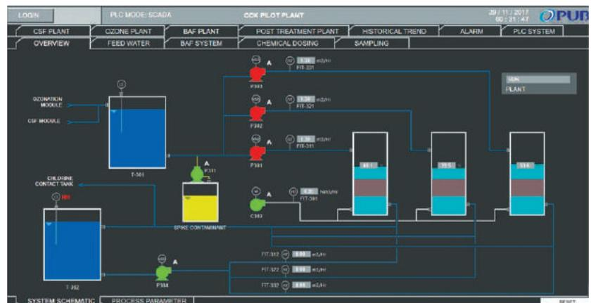
FIG. 2: A screenshot depicting the schematic flow of the BAF in the pilot plants
