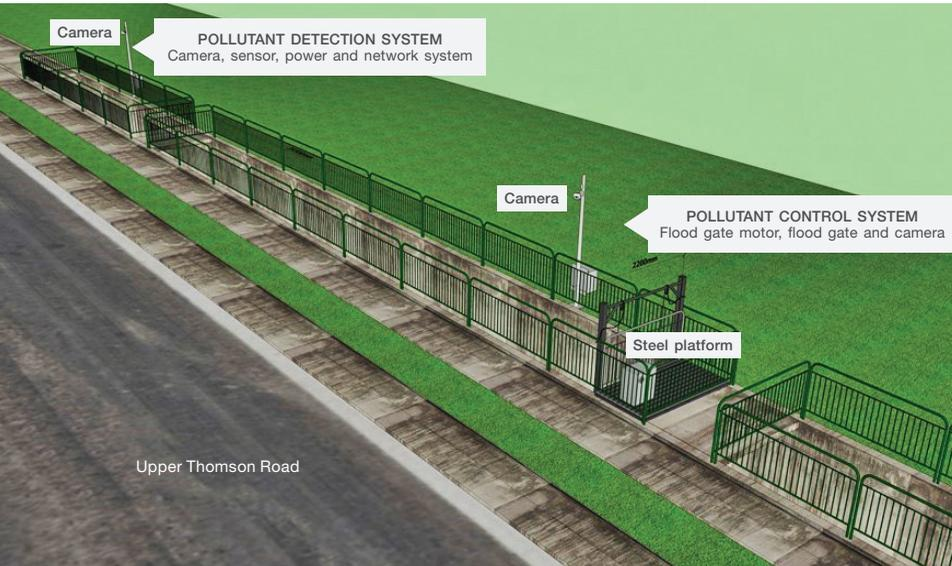
FIG. 1: Perspective view of the pollution detection and containment system
