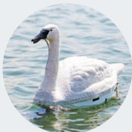
FIG. 3: A Smart Water Assessment Network (SWAN) robot performing water quality profiling
