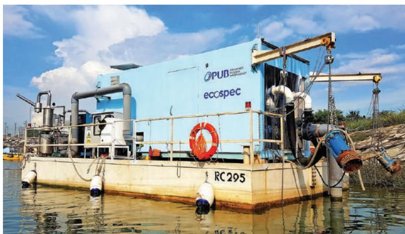
FIG. 1: The ultra-low frequency (ULF) treatment system onboard a floating pontoon in Serangoon Reservoir
