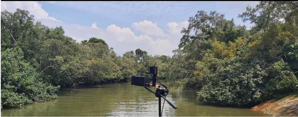
Eagle.pt, the contactless water quality monitoring sensor
