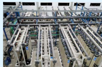
Treatment of surface water with dNF membranes for Dumai City, Indonesia
