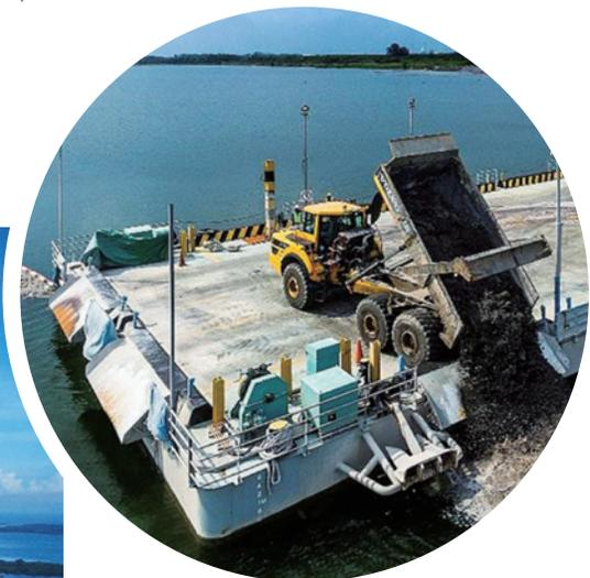
Figure 5. The offshore landfill at Semakau (left image) was created by building a 7km rock bund around Pulau Semakau, Pulau Sakeng and the surrounding waters, to create space where incineration ash generated from waste on the mainland is deposited (top image). This solution has a finite capacity. Photos credit: National Environment Agency
