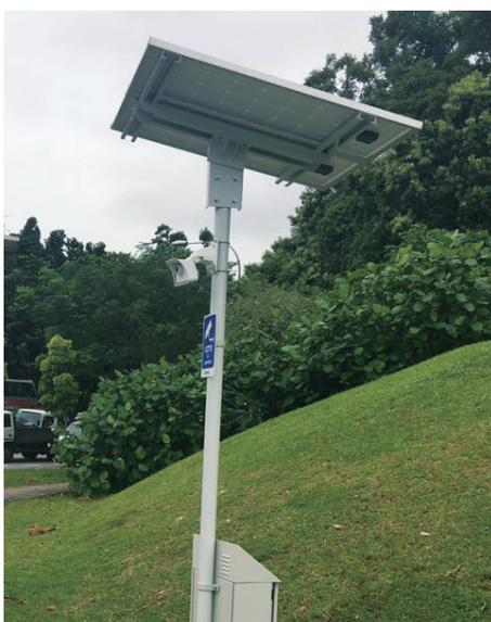
Figure 1. CCTVs are designed to record and monitor scenes. However, by harnessing advanced technologies, they can be also be used as a rain gauge.
